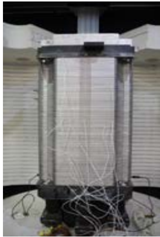
Current Pre-Commercial Integrated Manifold (PCI) Stack
