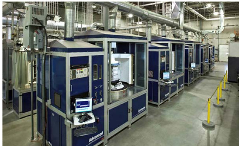
25kW Test Stands for Factory Acceptance Testing
